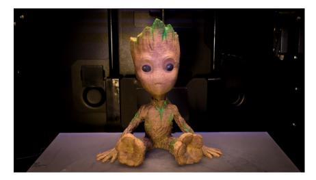
Downloading models from sites like thingiverse is a great way to get started with 3D printing. Above is a 3D model of Baby Groot that was downloaded and 3D printed using wood fill - a composite filament made of pla and wood fibers. The model was then painted.
